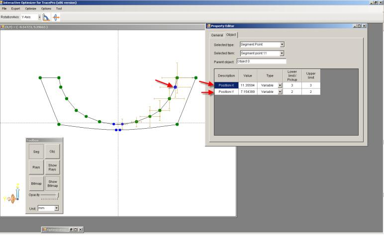
After selecting a point on the reflector the Property editor's Object tab allows to specify an exact value, the point as a variable with limits or a pickup to another point.
