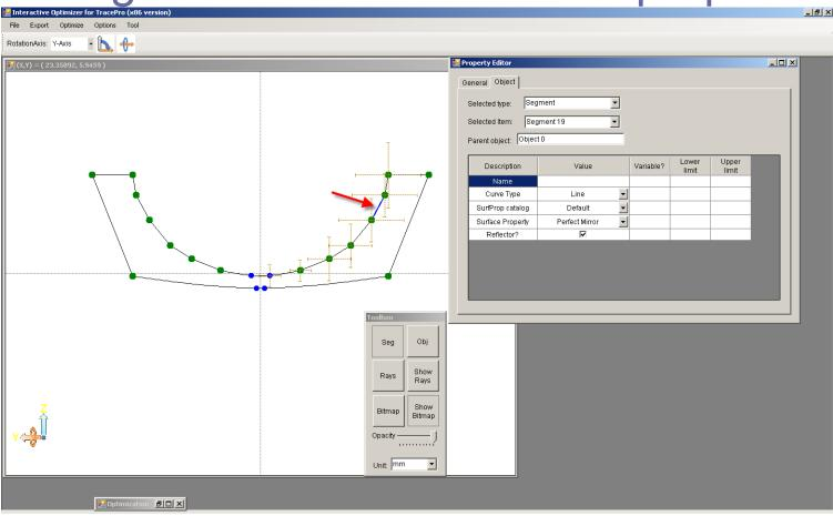
After selecting a segment point you can make it reflective or transmissive or specify a surface property from the TracePro database by selecting the line segment and selecting the value in the Surface Property portion of the Property Editor dialog.
