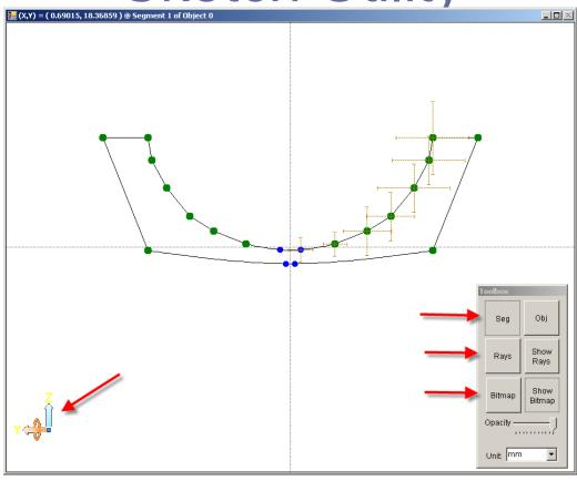
The main Toolbox of the optimizer allows you to digitize in a design, do interactive raytracing and bring in bitmaps to digitize sketches. In this example we are digitizing in a faceted reflector for a downlight with the reflector pointed down the Z axis.
