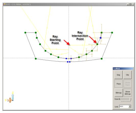
After selecting the Rays tool from the Toolbox you can interactively trace rays in the Optimizer Utility. You can then switch to the Seg Tool to move segment points so that you can quickly analyze and control angular ray control for each facet
