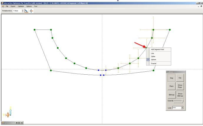
When the Seg tool is active, you can select any segment or add segments to your design. Shown is the capability to add a line or spline segment to your design
